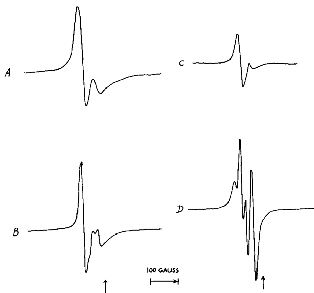
FIG. 4. EPR spectra of a mixture of \text{TiCl}_4 and \text{Al}(\text{C}_2\text{H}_5)_3 recorded at: (a) -130^\circ (1); (b) -50^\circ (1); (c) +70^\circ (1); (d) \text{CH}_3\text{CN} added, +25^\circ (0.4); markers at 3325 G (numbers in parentheses correspond to instrument gain).
